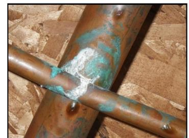
Water testing can help determine the corrosivity of your water.
